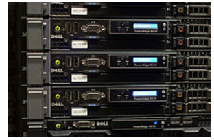
Rack-mounted 11th-generation PowerEdge servers
